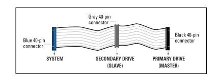
1. Connect the IDE Interface Cable to the Hard Drive(s).
